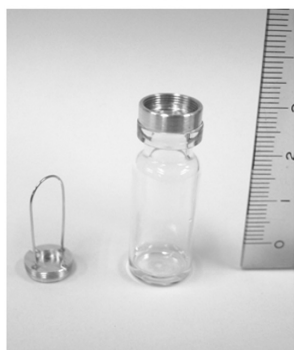
Fig. 1 Baseline for calorimetry at T=293 \text{ K} . Ampoules with 0.1 mL ASW were loaded into the measuring cylinder. Standard deviation was 7 nW. Photo shows the glass ampoule with aluminum alloy cap
